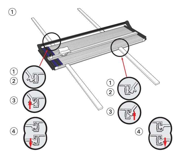
The Base Extension Arms are packed in pairs and can be fitted to either side of the Base. When large boards are cut on the machine they give the support necessary to keep the material flat for accurate cutting.
